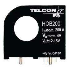
The HOB series are Open Loop Hall Effect Current Transformers covering the range of 25A to 400A. The product provides a voltage output which is galvanically isolated from the primary circuit. All contacts, including the primary are designed to be PCB mounted.
